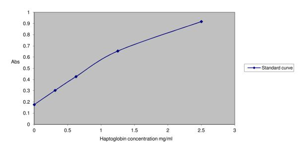
**Note:** An example of a typical standard curve is presented above. This should not be used in determination of haptoglobin.
